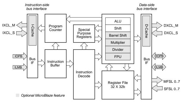
Figure 1-1: MicroBlaze Core Block Diagram
